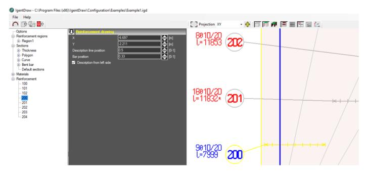
The program provides support for definition of reinforcement regions based on DXF background. The first step is to load the DXF file (**File / Import**). The DXF 12 file format is required at the moment. The program allows to load all or selected layers of a drawing. Once the drawing is loaded, layers visibility can be switched on / off freely. (**Options / Layers**). During DXF file loading, the unit of length in which the drawing is defined should be chosen.
