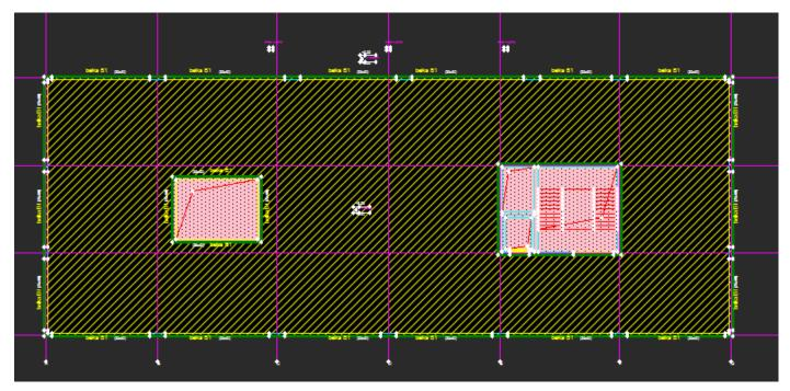
After switching on the Reinforcement option in the parameter window, we automatically get a drawing which, after setting the selected parameters (f. ex. hooks for bars), becomes the final drawing. The DXF background can be presented in a small scale in the parameter window as well as in the view window after selecting the icon "Full window viewer" on the toolbar. The project can be saved in the internal **igd** format. The last step is to export the
