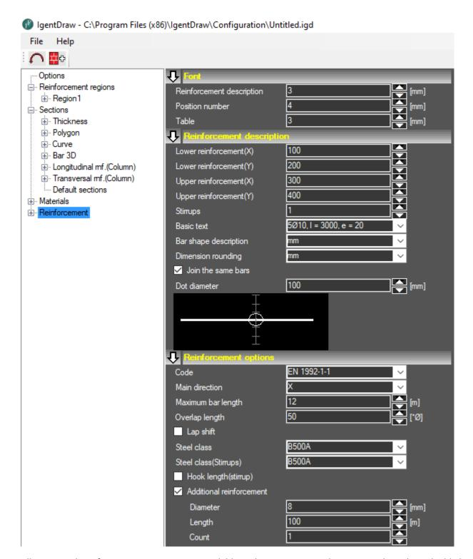
All generated reinforcement positions are available in the inspector window. Once selected, it is highlighted on the view. For each item the following parameters in the group **Reinforcement drawing** can be set:
