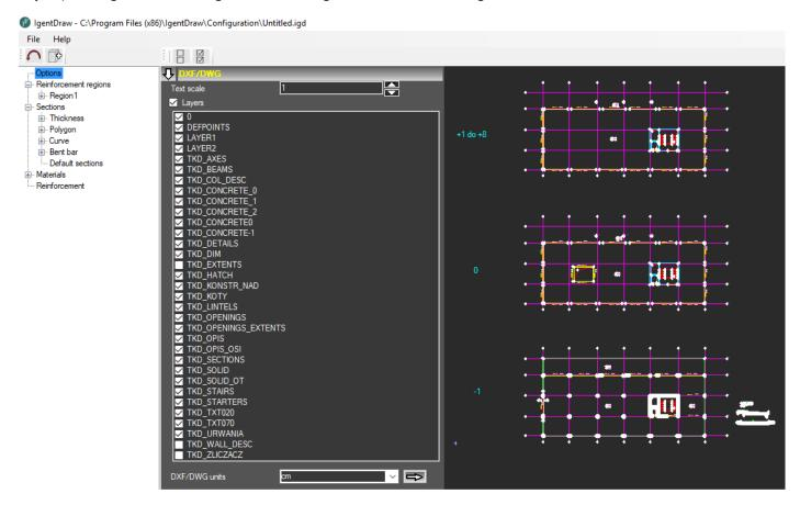
The regions are entered by clicking the **Poligon** in the **Sections** branch in the inspector window and selecting one of the two icons on the toolbar. These options allow to define the region by choosing a layer from the DXF file (automatic detection of closed contours), clicking inside the closed contour or by sequentially selecting the next contour vertices (clicking on the first or last point completes the edit).
