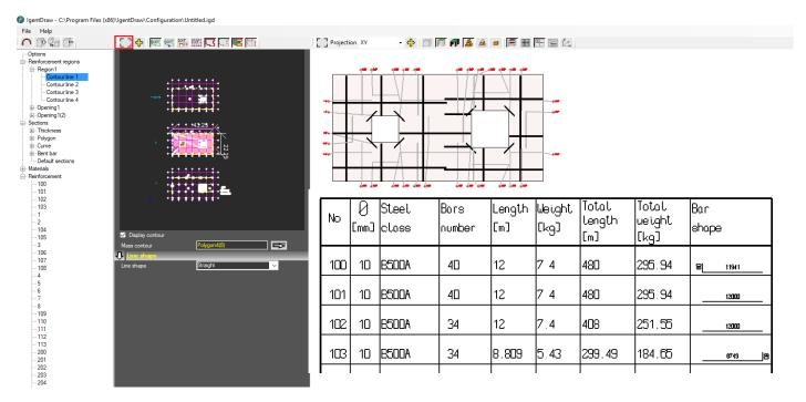
After selecting the Options item in the inspector window, parameters regarding column reinforcement can be set
